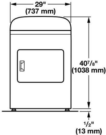
**NOTE:** Minimum height of leveling legs should be 1/2" (13 mm), or to match the height of the accompanying washer.
