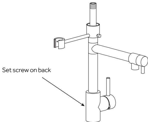
7. Attach the hose and spout spring to the faucet body. Apply a small amount of thread sealant, or plumber's tape, to the threading on the faucet body before attaching.
