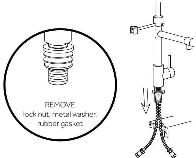
4. From beneath the sink, slide the rubber gasket back onto the faucet body, followed by the metal washer. Thread the lock nut back onto the faucet body using a basin wrench. Finish tightening by turning the two screws attached to the lock nut to the right.
