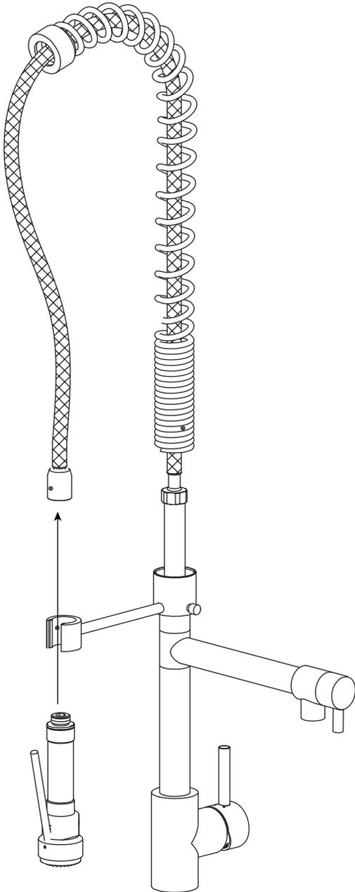
9. Once installation is complete, turn the main water supply back on from underneath your sink. Check for any leaks underneath.
