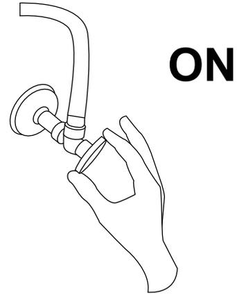
10. Remove the aerator from the main faucet spout using the provided removal tool. Turn the faucet on and ensure that there are no leaks. Check to ensure that both hot and cold water are running properly. Allow for the water to flow for approximately 60 seconds to remove any dust or sediment within the water lines. Reattach the aerator and turn on the sprayer. Allow the sprayer to run for another 60 seconds, and check for any leaks.
