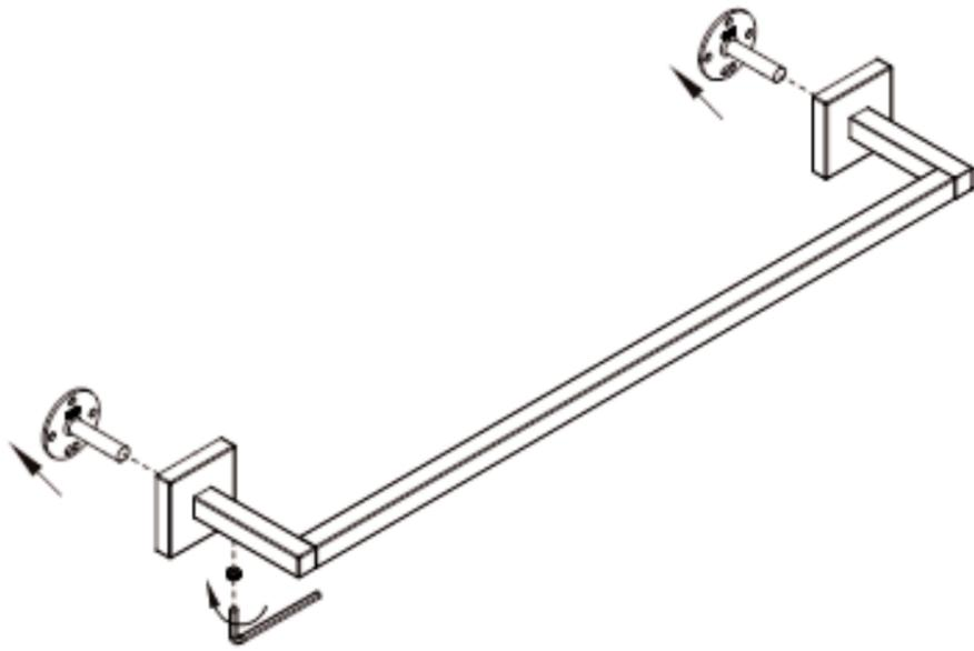
② ALIGN MOUNTING BRACKETS AND MARK LOCATION
