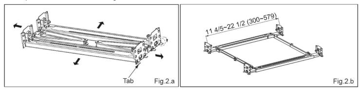
2. Secure one side of the suspension bracket assembly to one joist by drilling in the two (2) ST4x20 screws attached to the assembly as shown in Figure 3. Then adjust the length of the suspension bracket assembly to fit the spacing between joists and drill in the other two (2) tapping screws attached to the assembly.
