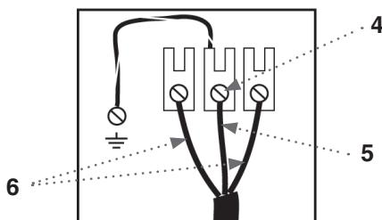
5. Connect ground (center) wire of power supply cord to the center, silver-colored terminal screw. Tighten screw.
