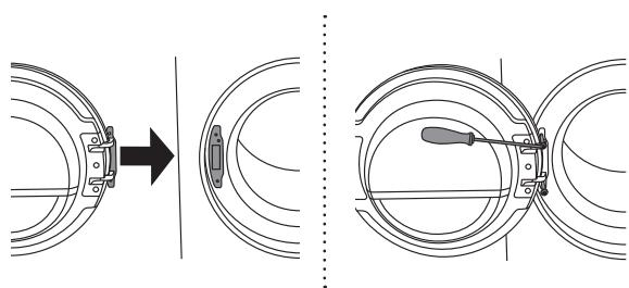
**10** Replace the door on the door hinge and fasten the screws.
