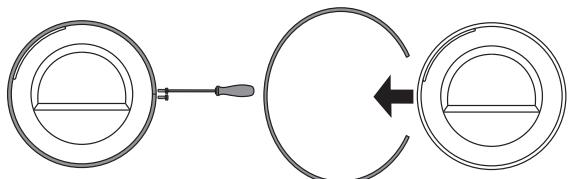
**7** Undo the door ring and remove it temporarily.
