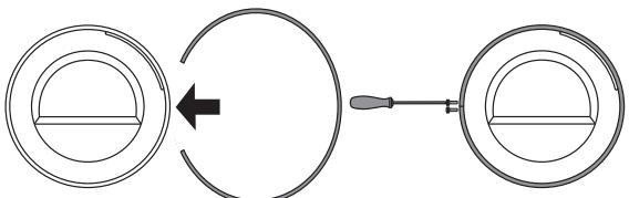
**9** Rotate the door ring by 180°, install it onto the door, and fasten it with screws.
