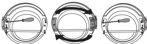
**6** Undo the door hinge assembly (left) and the door latch assembly (right), switch their positions, and replace the screws (door hinge assembly to the right-hand side, door latch assembly to the left-hand side).
