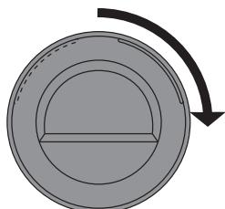
**8** Rotate the door glass cover by 90° so that the sign indicating the opening of the door is on the other side.
