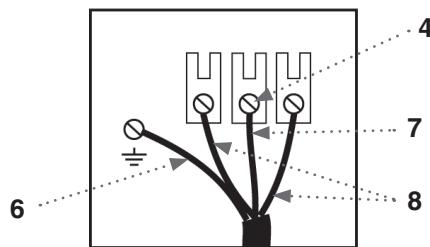
5. Remove ground wire (green with yellow stripes) from external ground connector screw and remove from center terminal block.
