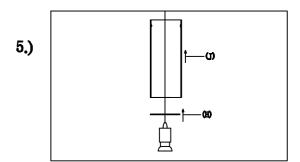
Step.5: Run socket and wire through second ring (H) and outer glass (J) as shown.
